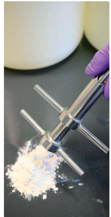
Sample being discharged from a Standard Slot Sampler without a Bottle Holder
